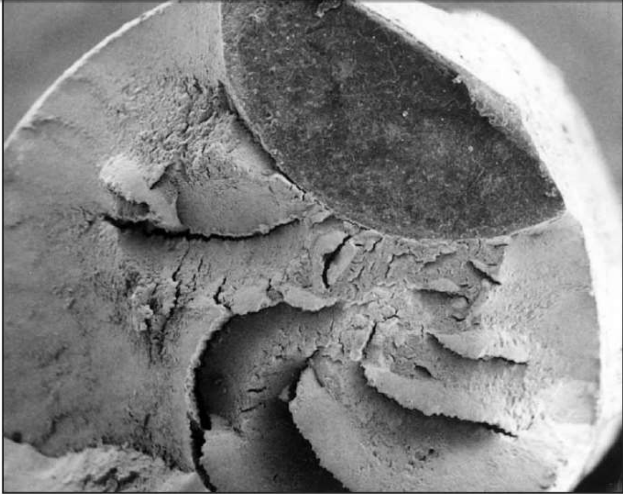
Fig. 15: A fatigue crack starting at the point of contact with a sheave. Obviously the crack propagated concentric to its point of initiation. The crack only became visible after destroying the strand in a pull test.
